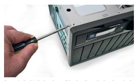
Access to the interior is only possible when the main chassis casing has been removed.
