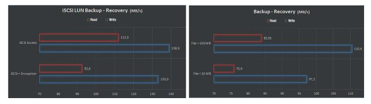
Backup and recovery on iSCSI LUNs can reach 138.9MB/s read and 112MB/s writing speeds, which matches what we recorded during the tests of the RDX unit separately inside a Windows Server workstation.
