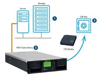
As a secondary backup target, the NEO tape libraries offer automated backup processing on a second media beside disk. As already mentioned, backups are already protected against crypto lockers and viruses even if an LTO tape media resides in the drive. To build the final stage of the 3-2-1 backup strategy, a third backup copy should be created on a second LTO media which should be ejected after the backup is complete to store off-site.
