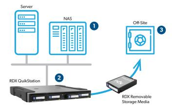
Due to its removable media design, QuikStation can also play the role of the tertiary backup device. A backup copy to a second RDX media can be ejected and placed off-site after the backup job is finished.
