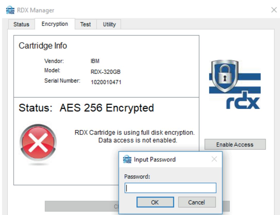
If automatic decryption is not enabled, a password is required to access data on the RDX media
